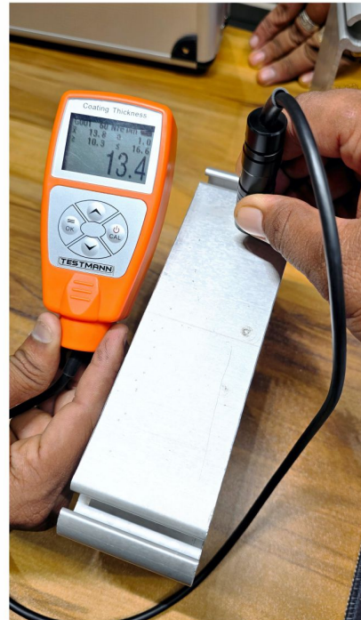
Aluminum Anodize-Layer Thickness 10 \mu m To 15 \mu m
